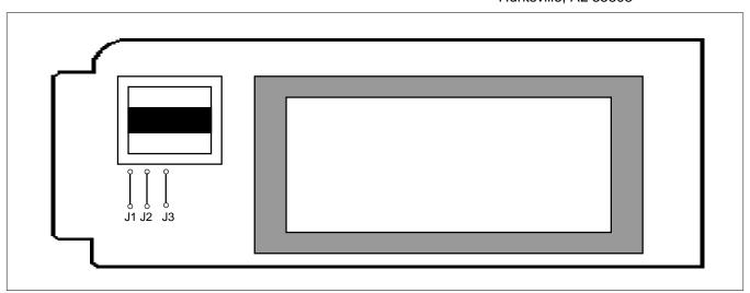
FIGURE 4. U-Repeater Powering Module Option Locations
